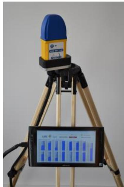
*EME Spy 140 +Tablet PC mounted on wood tripod*
